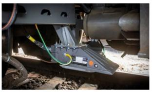
ETCS sensor DRS0551 on a 362 series locomotive
