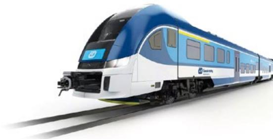
**20 nine-car push-pull non-traction units for** international and domestic long-distance transport. The maximum speed of the units will be 230 km/h, with the capacity of 555 seats. Deployment is expected on the lines Prague - Ústí nad Labem - Dresden - Berlin - Hamburg and Prague - Brno - Bratislava – Budapest. The units will be delivered in 2024-2026.
